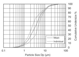
Cumulative % particle mass of sodium fluoride under size
