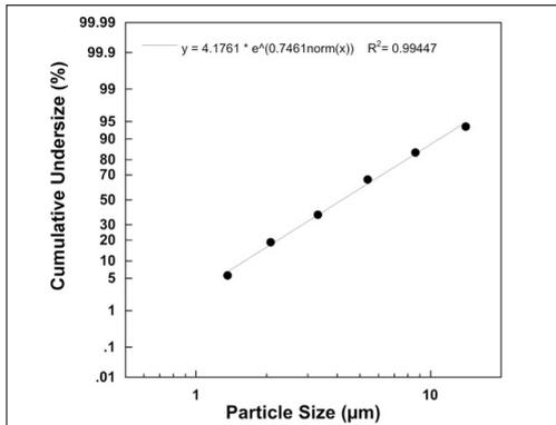
Measurements were performed using a sodium fluoride solution with a “Next Generation Impactor” (NGI). The diagram may therefore not be applicable to suspensions or highly viscous medications. You can obtain more detailed information from the manufacturer of your medication.
